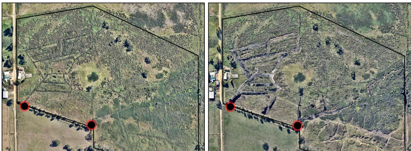
High resolution aerial imagery before and after the completion of peat channel packing (backfilling) in April 2017. Note the surface water visible (black) in the second image, from permanent groundwater discharges.
