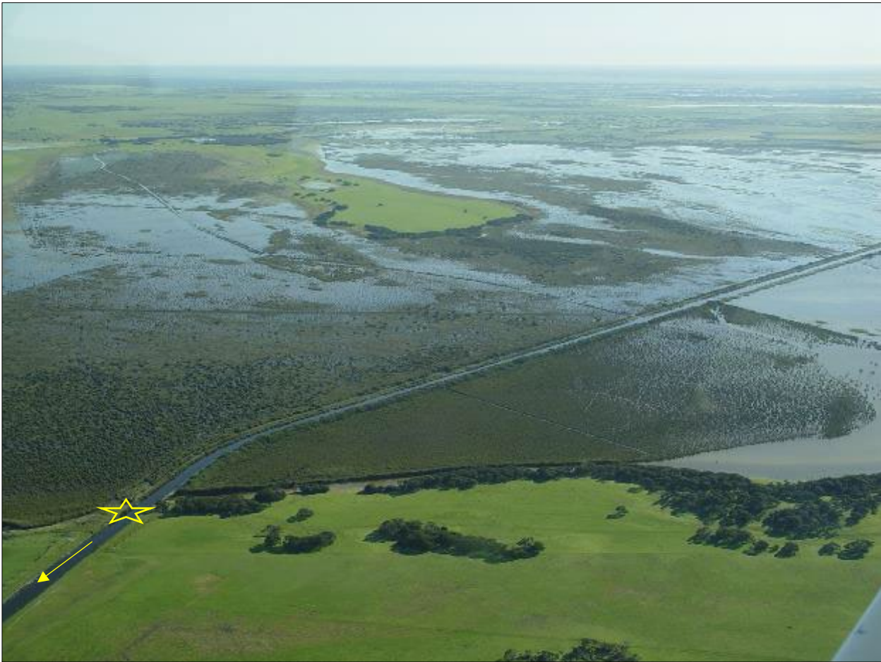
Figure 12. Proposed location of a regulator on Drain L (yellow star) to manage water levels in Lake Hawdon North. The direction of flow in the drain is also shown (yellow arrow) (photo: Ben Taylor).
