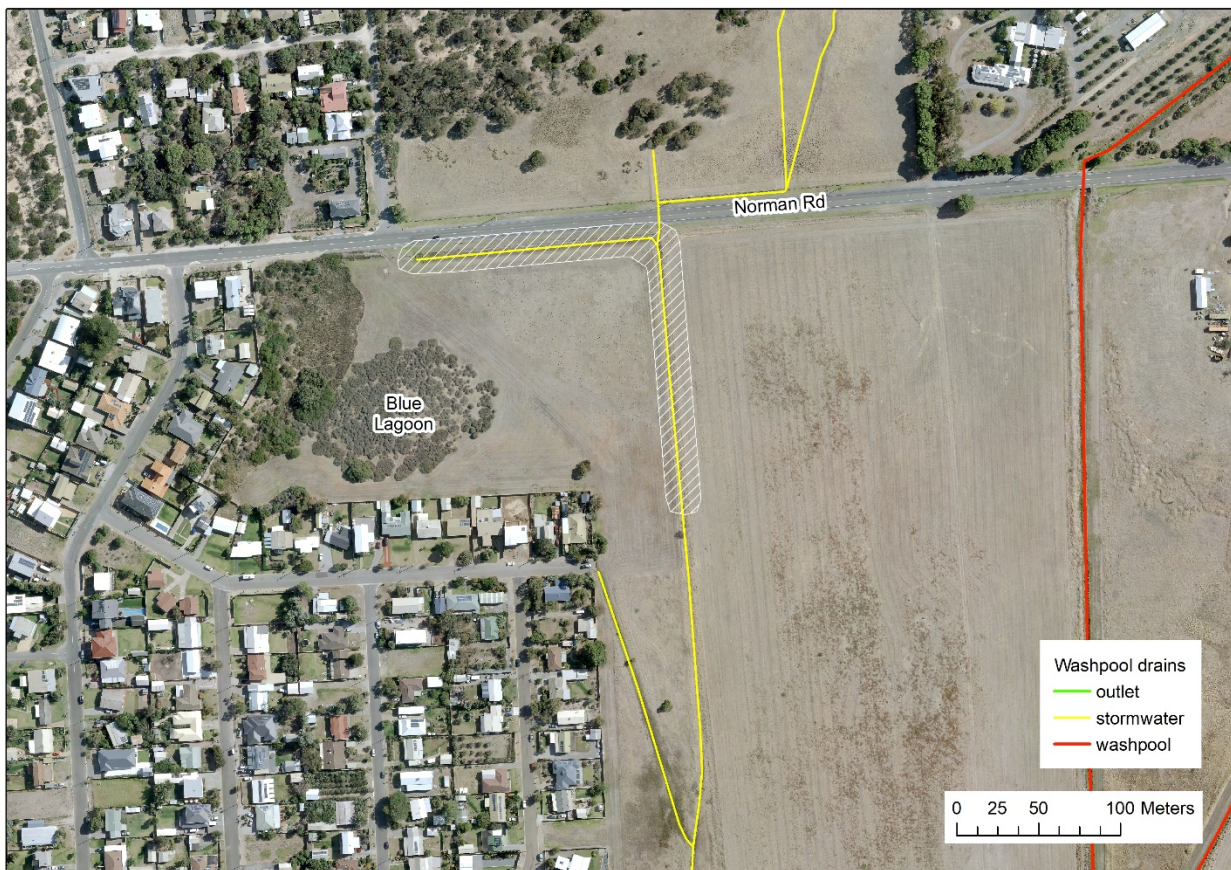
Figure 53. Section of drain near Blue Lagoon proposed for backfilling (white cross-hatching).
