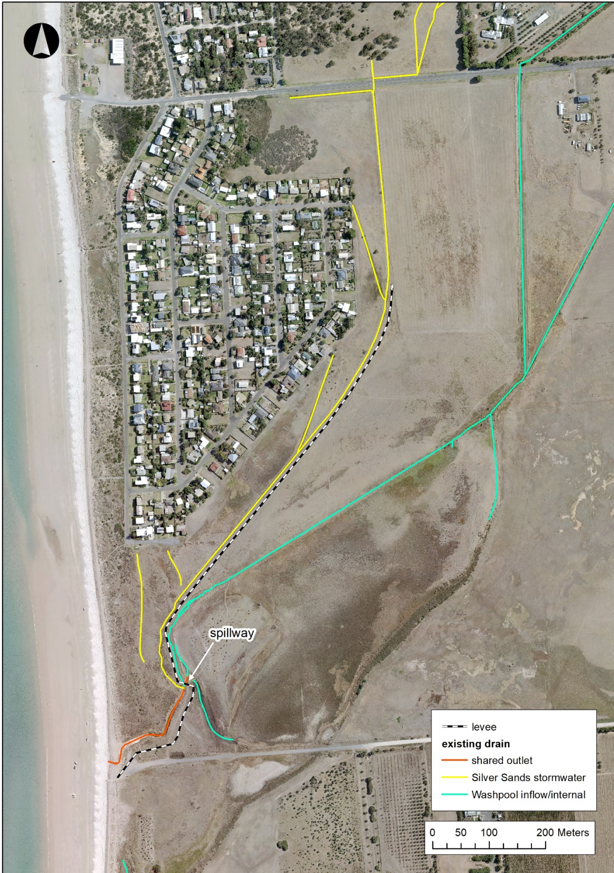
Figure 40. Proposed levee alignment.
