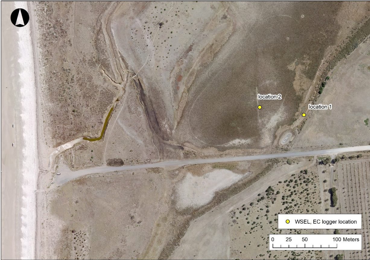
Figure 27. Water surface elevation (WSEL) and conductivity (EC) logger locations established by NGT in the Washpool.
