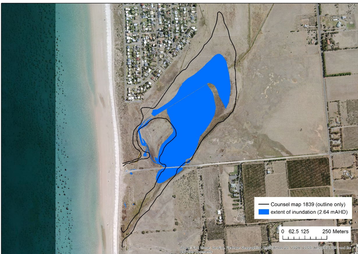
Figure 46. Extent of inundation in the Washpool at CTF if accumulated sediment were removed (Option 3) but existing concrete weir was maintained as sill.
