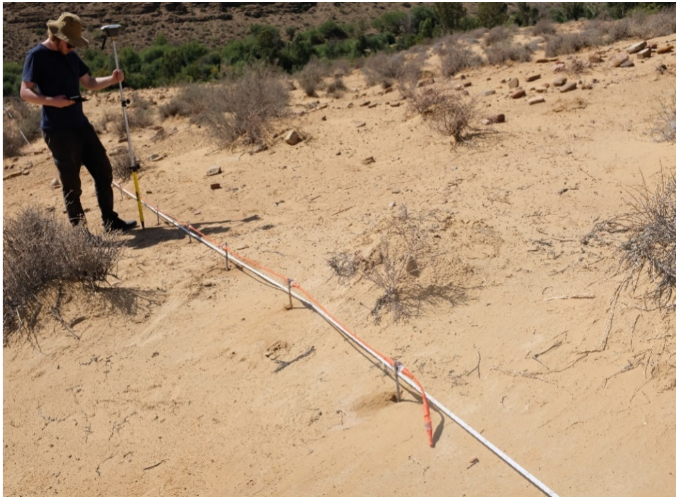
Figure 41. Electrical resistivity tomography in progress (photo courtesy of Dr Ian Moffat, Flinders University).
