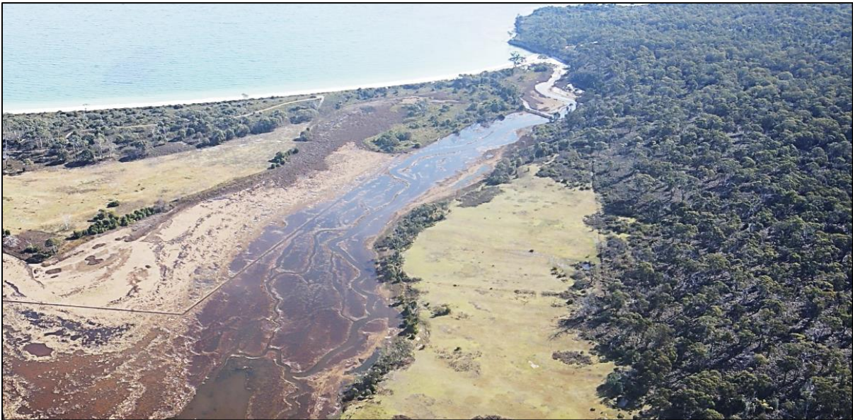
Figure 35. The outlet to the sea at Burdens Marsh, showing the constriction caused by the levee and gate system.
