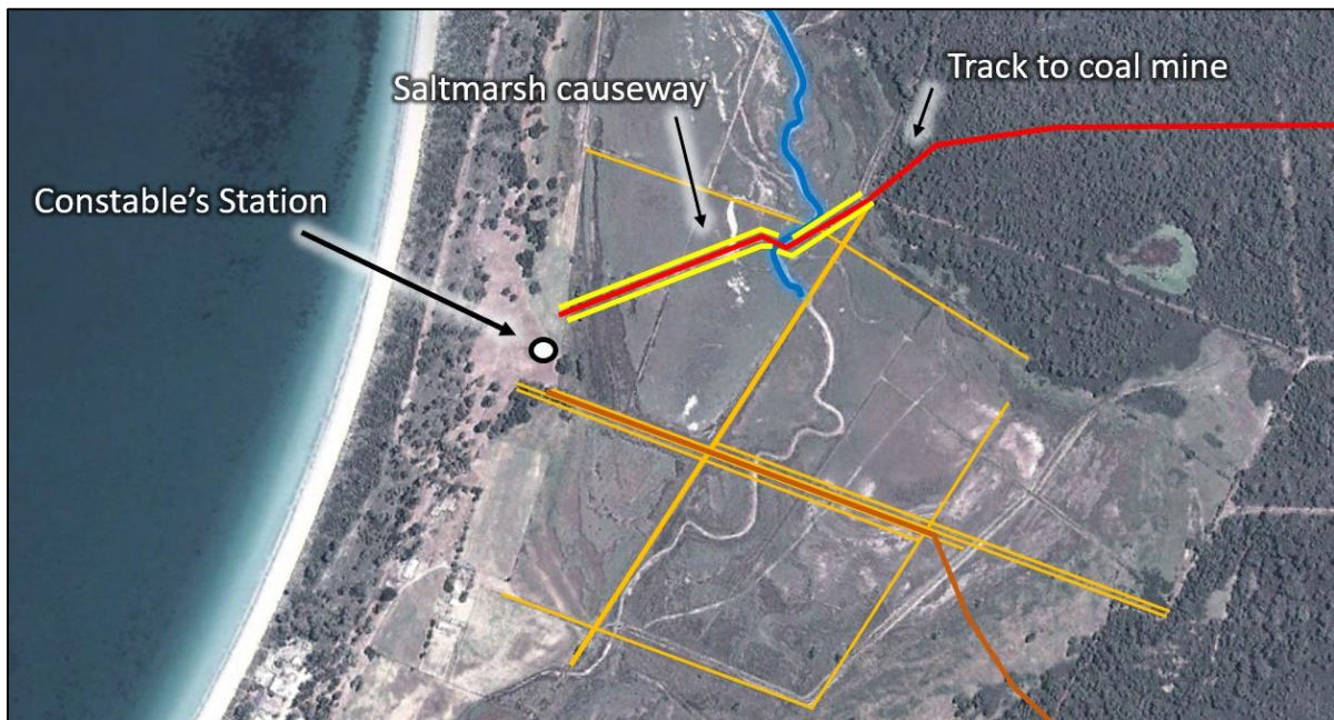
Figure 13. Works that date to the mid-1830s through the saltmarsh, providing more direct access to the coal mines. The red line indicates the location of the new track, and the yellow lines are the ditches that were dug either side to gain the material required to create the causeway. Earlier works are marked in orange (drains) and brown (roads).
