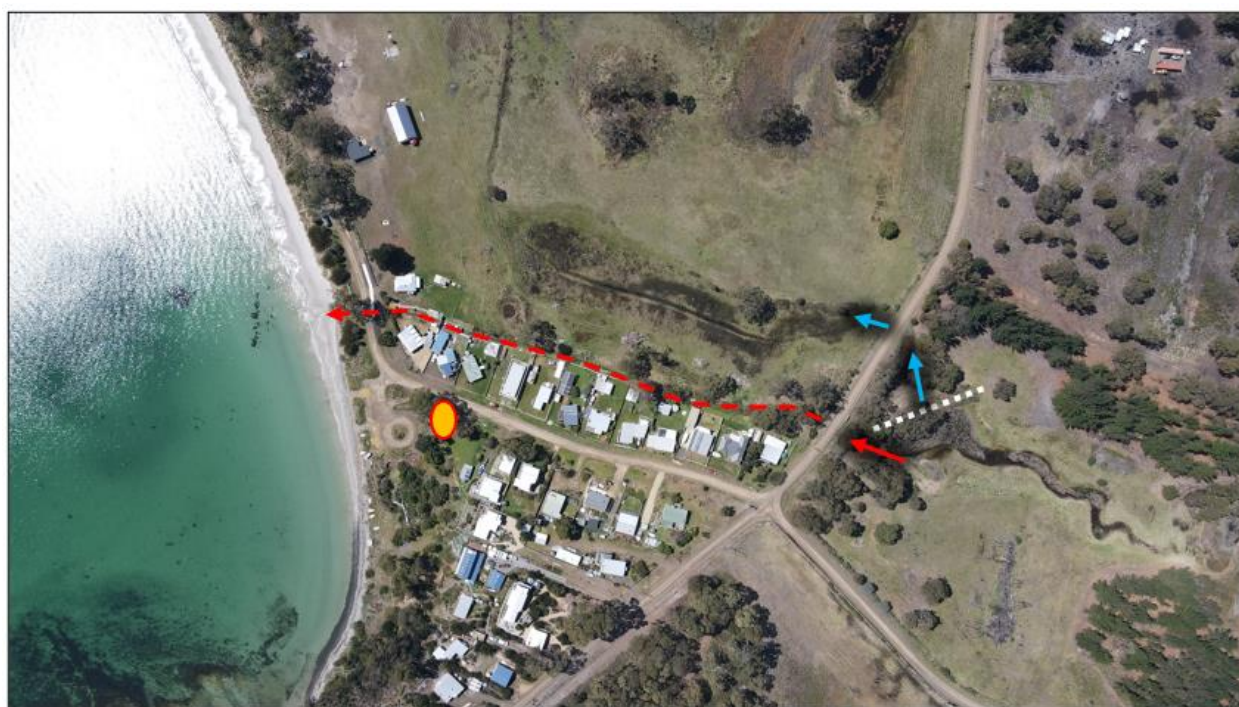
Figure 22. The original flow direction of the southern catchment into Burdens Marsh (blue arrows), was banked off (white dashed line), and this catchment has been diverted (red arrow) via an artificial bypass drain to the sea (red dashed line) since the early 1900s. The approximate location of the old waterhole/trench for the timber mill is shown in the orange circle. Photo: Mark Bachmann
