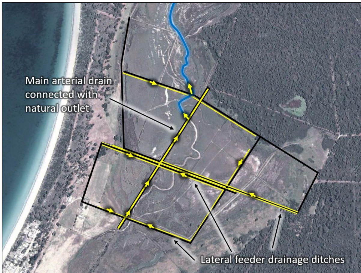
Figure 8. Likely drainage configuration established by Gellibrand before 1834. Paddock boundary fences are marked in black, while inferred locations of original drains based on modern observation and LiDAR data are marked in yellow. The saltmarsh outlet is marked in blue and yellow arrows indicate direction of flow.
