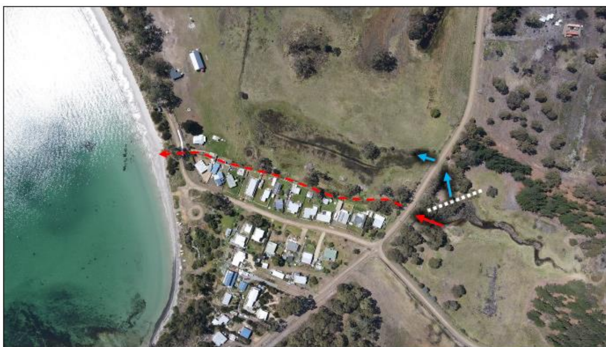
Figure 39. The original flow direction of the southern catchment into Burdens Marsh (blue arrows), has been banked off (white dashed line), with this catchment now diverted (red arrow) via an artificial bypass drain to the sea (red dashed line). Photo: Mark Bachmann
