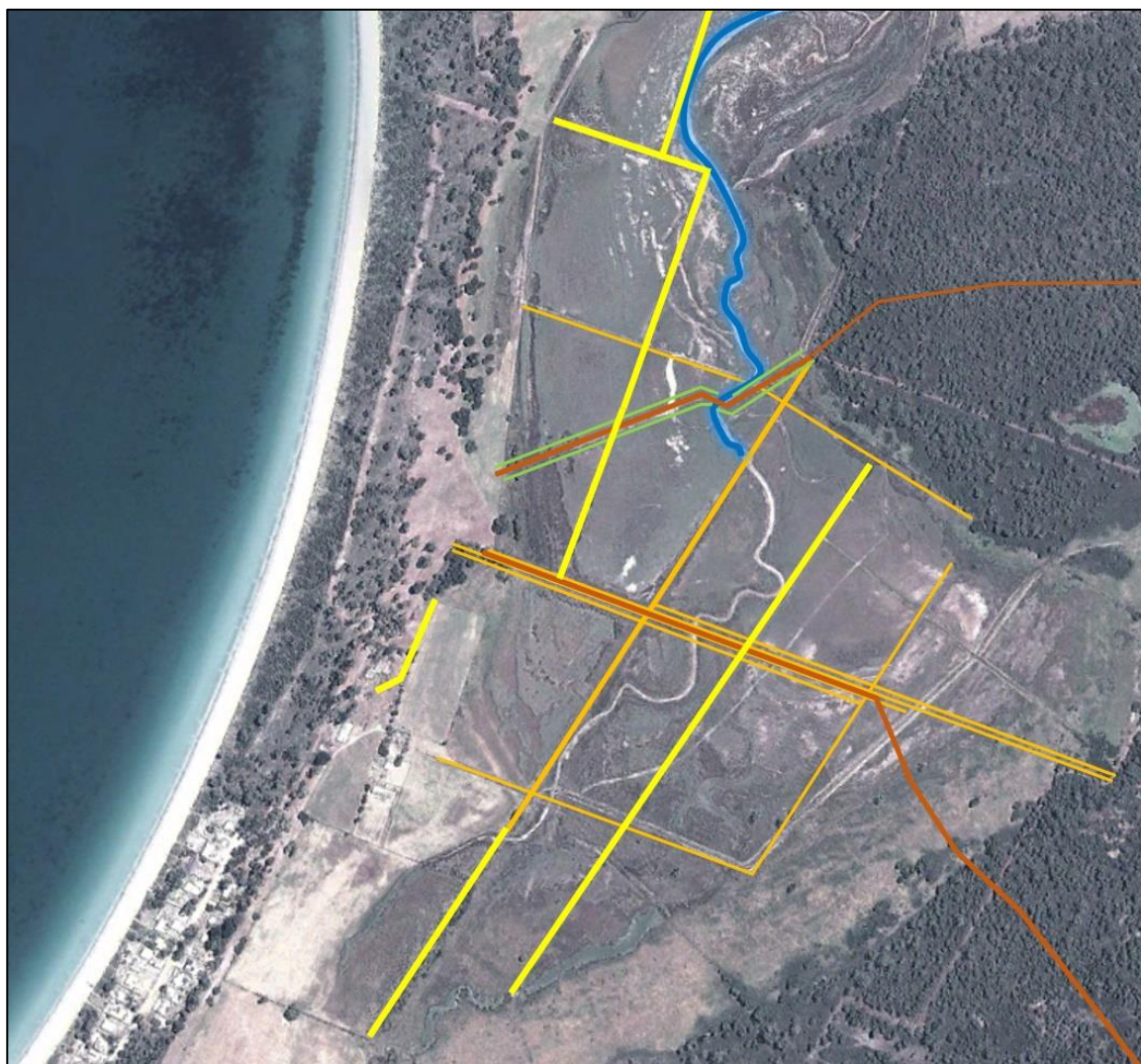
Figure 19. Summary of drainage works prior to the 1940s in Burdens Marsh. The orange lines are the original pre-1834 drains, while the yellow lines are the additional drains probably excavated by convict labour between 1834 and 1847. After 1878, Jacob Burden likely reactivated all pre-existing drains (which were unlikely to have been maintained since their construction). The tracks from the 1830s are marked brown and the green lines are the ditches either side of the 1830s coal mine crossing.
