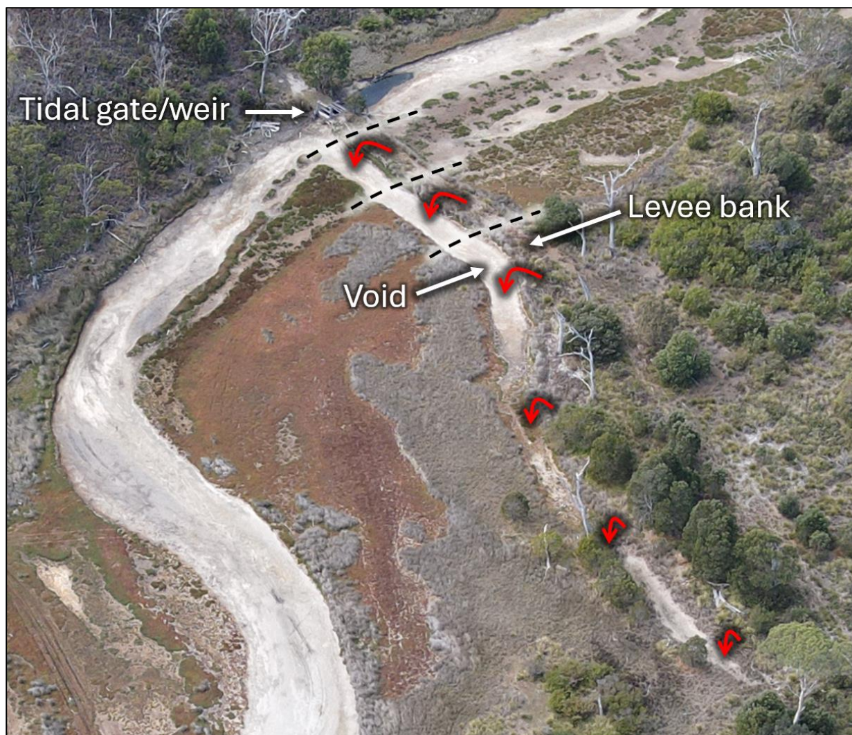
Figure 55. The remedial earthworks required at the ocean outlet from Burdens Marsh. See text for explanation of notations. Photo: Mark Bachmann.
